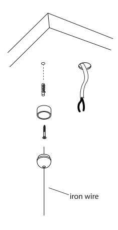
Fissare la lampada tramite i cavi e i gripper Fix the lamp with the wire gripper
